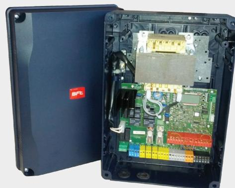
Control panel for one or two 24v operators for swing gates. The main features include removable terminal blocks with new standard colour-coding, simplified scenario based programming with display and incorporated dual channel receiver, D-Track anti-crushing system, slowdown during opening and closing and electronic self learning.
